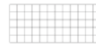
60 Tile Assembly 1 row of 6x6 tiles 1 row of 6x12 tiles 1 row of 6x18 tiles
